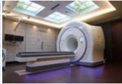
TomoTherapy (High-precision radiotherapy device)
